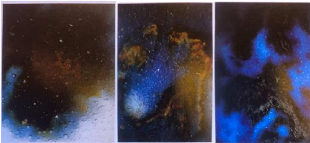
Figure 11 Surface effect of blue colour on Xuande qinghua: (left) brown-green crystalline spot; (middle) brown-yellow crystalline spot; (right) Iron brownish crystalline spot
